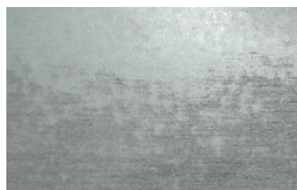
Z275 sample showing severe degradation after 600 hours at 350 °C
